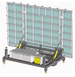
Automatic trolley to transport big glass sheets from one production unit to another, with hydraulic lifting system from 0° to 90 °.
